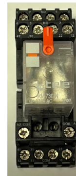
Tripping Relay OPEN
